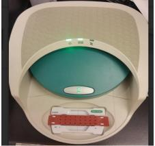
5. After droplet formation is complete, the resulting droplets will be available in the top row of the cartridge, labeled "Droplets", and should appear cloudy. Using a multi-channel P200 pipette set to 40 µL, slowly aspirate up the droplets and deposit into a fresh Bio-Rad 96 well plate kept in a
