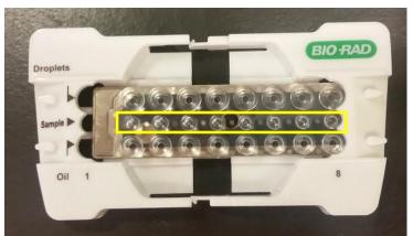
hold 8 samples. For 96 samples, 12 DG8 cartridges can be pre-loaded with sample and oil prior to droplet generation in step 4, below.
